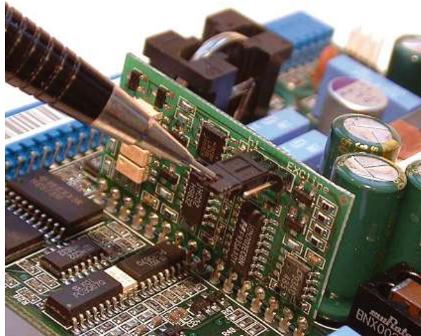
The jumper for selecting EXOline/hEXOline.
